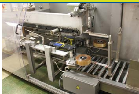
“Marchesini” Case Packer and Palletiser, Model MCP840, Year 2000, setup for tape sealing and complete with a HSAjet inkjet printer fully guarded and full controls.
