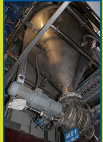
Bag unloading room, complete with 2 x "Flexicon", Bulk Bag Unloaders, each setup in a mild steel frame with electric hoist and trolley. Units complete with power cincher, bag activators, s/s hopper with agitator and vibrator. Safe working load of 1500kg, also included 2 x "Wilden" M8 Diaphragm Pumps, "DCE Vokes", dust collector and Rapid Roller Door
