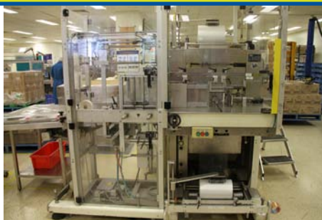
“Pester” Heat Shrink Tunnel and Collator, 200mm wide x 2100mm long infeed conveyor, Pewo Pack 450 SN stacking type collator and sleeve wrapper, 420mm wide Pester Heat Shrink Tunnel, gravity out-feed conveyor.
