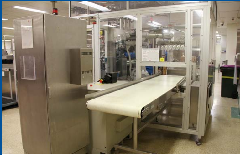
“Nordenmatic”, Tube Filler, Model 2002, complete with ABB Robot Model IRB 2400 M98 tube loader, 2 filling heads, suitable for 3 products/colours in the one tube, hot air sealing with leak detection system, Year 2002
