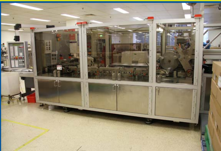
“Nordenpac” Cartoner, Model 2002, setup with infeed conveyor with push type transfer, automatic carton loading machine / erection station, Nordson Vista Gluing system, fully guarded, fully adjustable and automatic, full controls
