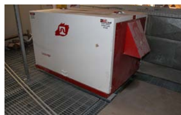
Bag unloading room, complete with "Flexicon" Bulk Bag Unloader, mild steel frame with electric hoist and trolley, power cincher, bag activator, S/S hopper with vibrator, deflator, S/S rotary valve. SWL 1500kg, also included roots type blower DCE Vokes dust collector and Rapid Roller Door
