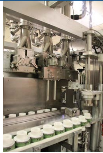
“Nordenmatic”, Tube Filler, Model 2002, complete with ABB Robot Model IRB 2400 M98 tube loader, 2 filling heads, suitable for 3 products/colours in the one tube, hot air sealing with leak detection system, Year 2002
