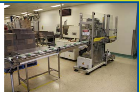
“Pester” Heat Shrink Tunnel and Collator, 200mm wide x 3300mm long infeed conveyor, Pewo Pack 450 SN stacking type collator and sleeve wrapper, Pester Heat Shrink Tunnel
