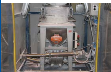
Bag unloading room, complete with "Flexicon" Bulk Bag Unloader, mild steel frame with electric hoist and trolley, power cincher, bag activator, S/S hopper with vibrator, deflator, S/S rotary valve. SWL 1500kg, also included roots type blower DCE Vokes dust collector and Rapid Roller Door
