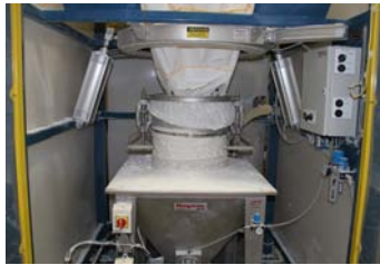
Bag unloading room, complete with 2 x "Flexicon", Bulk Bag Unloaders, each setup in a mild steel frame with electric hoist and trolley. Units complete with power cincher, bag activators, s/s hopper with agitator and vibrator. Safe working load of 1500kg, also included 2 x "Wilden" M8 Diaphragm Pumps, "DCE Vokes", dust collector and Rapid Roller Door
