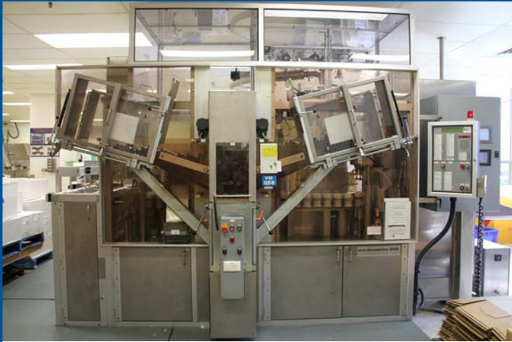
“Nordenmatic”, Tube Filler, Model 2002, unit is setup with automatic tube loader, 2 head fill, speed of 200 tubes per minute, control panel, high frequency sealing head with controller.
