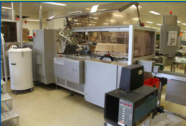
“Nordenpac”, Cartoner, “ Model 2002, unit is setup with fully automatic infeed conveyor, automatic carton erector, Nordson Hot Gluing unit, fully guarded, fully adjustable, full control panel, rejection station, and complete with transfer conveyor
