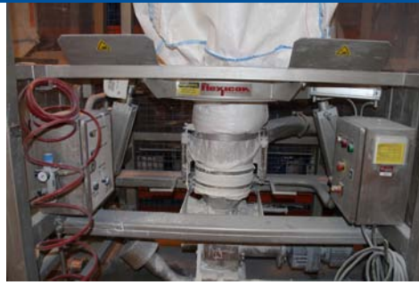
"Flexicon", Bulk Bag Unloader, setup in a stainless steel adjustable mobile frame for forklift loading of bulk bags. Unit complete with power cincher, bag activators and stainless steel rotary valve suitable for vacuum transfer. Safe working load of 1500kg, 2 available
