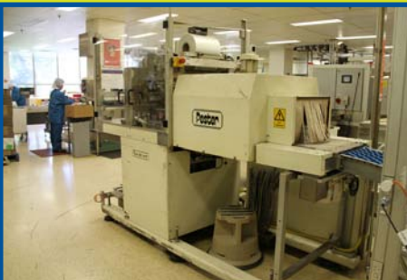
“Pester” Heat Shrink Tunnel and Collator, 200mm wide x 2100mm long infeed conveyor, Pewo Pack 450 SN stacking type collator and sleeve wrapper, 420mm wide Pester Heat Shrink Tunnel, gravity out-feed conveyor.
