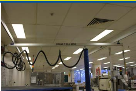
2 x VacuEasyLift, Vacuum Bag Lifter, Model 120, Max capacity 40kg, 6mtr overhead gantry
