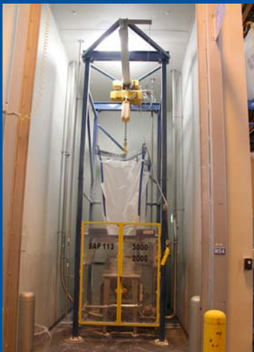
Bag unloading room, complete with 2 x "Flexicon", Bulk Bag Unloaders, each setup in a mild steel frame with electric hoist and trolley. Units complete with power cincher, bag activators, s/s hopper with agitator and vibrator. Safe working load of 1500kg, also included 2 x "Wilden" M8 Diaphragm Pumps, "DCE Vokes", dust collector and Rapid Roller Door
