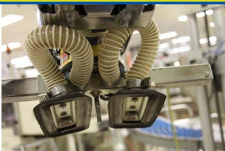
2 x VacuEasyLift, Vacuum Bag Lifter, Model 120, Max capacity 40kg, 6mtr overhead gantry
