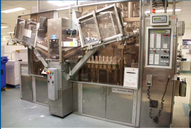
“Nordenmatic” Tube Filler, Model 2002, unit is setup with twin automatic tube loaders, 2 head fill, suitable for 3 different products/colours in one tube, Hot air sealing, full controls
