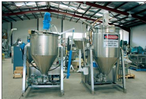
1. JACKETED VACUUM MIXING VESSEL "Fryma" 2. VACUUM MIXING VESSEL "Fryma"
