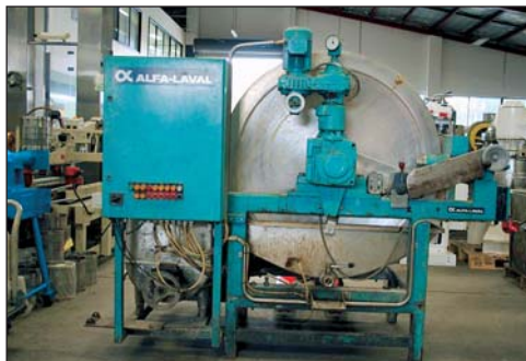
97. ROTARY VACUUM FILTER "Alfa Laval"
